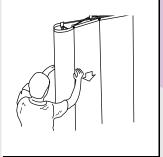
Slowly run your hands down the sides of the panel, attaching magnetic strips to the channel bars and straightening as you go.
