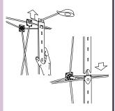
Mount top channel bars (with lights attached) to frame by aligning hole in channel bar over panel pegs on top hub and sliding up. Once top of channel bar is in place, slide channel bar down onto bottom hub to secure.
