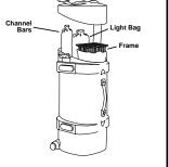
Collapse frame, pack in bag and insert into Case A. Pack lights in bag and pack in Case A next to channel bar bag as shown
