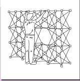
With the frame fully expanded, begin to lock the yellow spacer bars. Start with the spacer bars in the center area of the frame, then work toward the outer spacer bars.
