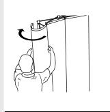
Lift end panel and guide front notch of plastic plate over front peg. Hook the other side on the panel peg at the back of the frame
