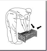
Continue pulling up and outward until the frame is fully expanded. Spacer bars should be close enough to each other to allow for a connection.
