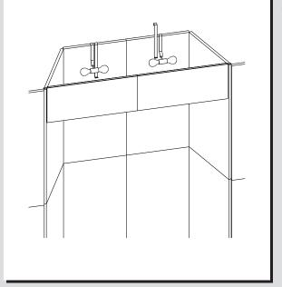
Attach H2 or H3 header to unit. Hang a pair of diffuser brackets from the top of the backwall adjacent to the light fixtures.
