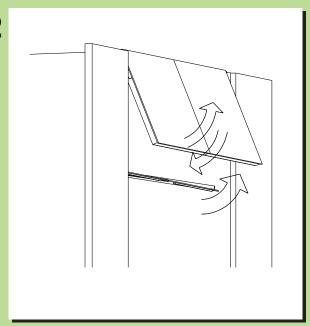
Swing header forward slightly, and raise diffuser. Lower diffuser so plastic strip on bottom of front edge fits inside the channel on the bottom of the header.
