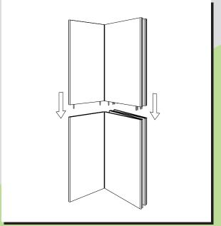
Lift upper panels onto bottom panels. Insert pegs in holes in bottom panels.
