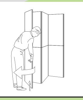
Open backwall to desired configuration. Push on bottom of system only. Maintain right angle on one panel to ensure stability.
