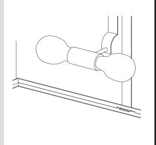
Hang the left half of the diffuser from the left diffuser bracket. There is a slot in the diffuser's extrusion to accept the bracket.
