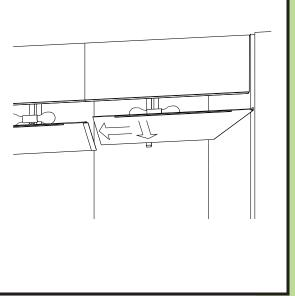
Hang the right half of the diffuser from the right bracket, and insert edge into the "H" moulding which is glued to the left half.
