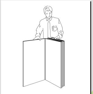
Position bottom panels (holes up). Adjust panels so edges are even. Partially open one panel for stability.
