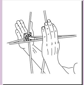
Ensure that spacer bars are fully engaged and locked.
