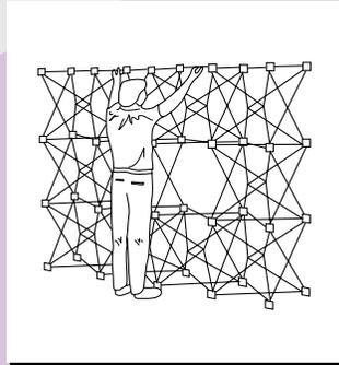
With the frame fully expanded, begin to lock the yellow spacer bars. Start with the spacer bars in the center area of the frame, then work toward the outer spacer bars.
