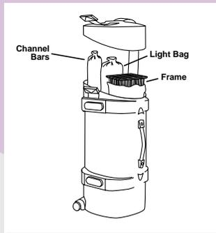
Collapse frame, pack in bag and insert into Case A. Pack lights in bag and pack in Case A next to channel bar bag as shown.
