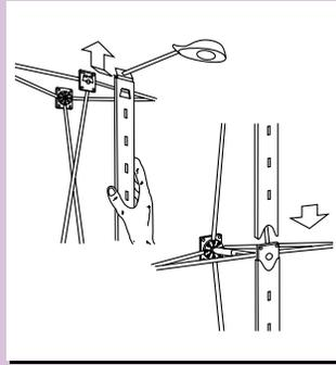
Mount top channel bars (with lights attached) to frame by aligning hole in channel bar over panel pegs on top hub and sliding up. Once top of channel bar is in place, slide channel bar down onto bottom hub to secure.
