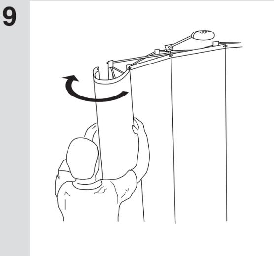
9 Lift end panel and guide front notch of plastic plate over front peg. Hook the other side on the panel peg at the back of the frame.
