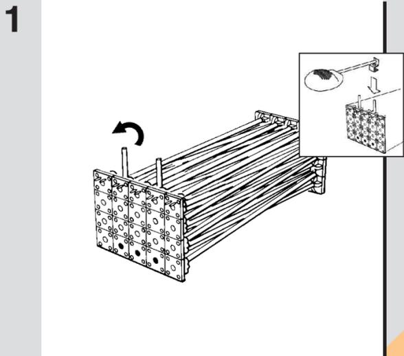
1 Remove frame from case and place on floor. Stand in front of unit with the yellow dots on bottom and facing you. Lift light posts and attach lights.
