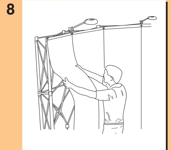
8 Release the panel, allowing it to attach magnetically to the channel bars. Straighten each panel by aligning it to the center of the channel bar slots.
