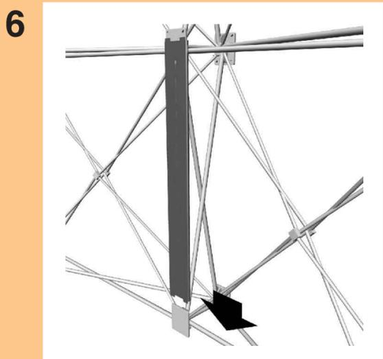
6 Line up the bottom of the channel bar over the lower hub and slide down to secure.
