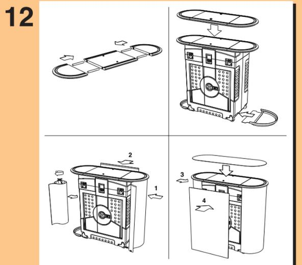
12 4300 Case Conversion: Assemble top and secure to case using a coin to tighten the two fasteners. Slip an end tray under both sets of wheels. Store panel liners and bags under table top overhang. Attach panels in numbered order as shown.
