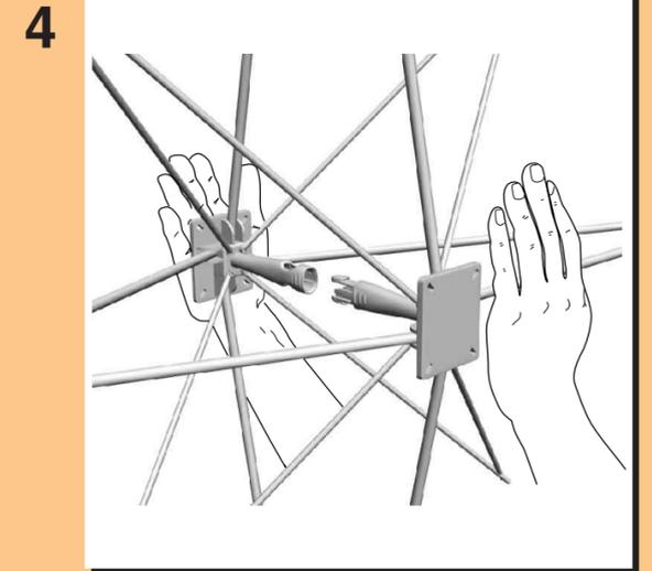
4 Ensure that spacer bars are fully engaged and locked.
