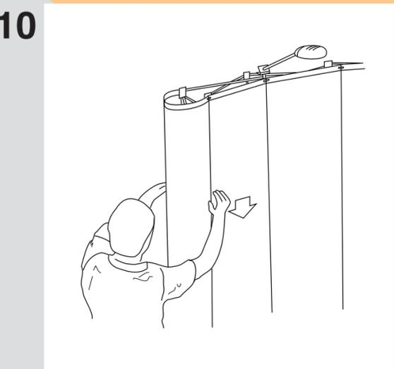
10 Slowly run your hands down the sides of the panel, attaching magnetic strips to the channel bars and straightening as you go.
