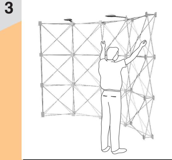
3 With the frame fully expanded, begin to lock the red spacer bars. Start with the spacer bars in the center area of the frame, then work toward the outer spacer bars.
