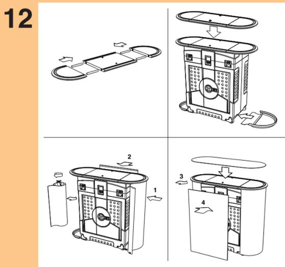
12 4300 Case Conversion: Assemble top and secure to case using a coin to tighten the two fasteners. Slip an end tray under both sets of wheels. Store panel liners and bags under table top overhang. Attach panels in numbered order as shown.
