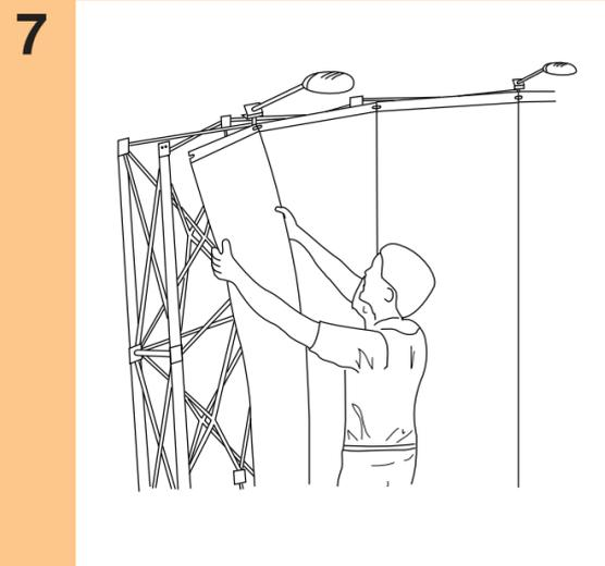
7 Grasp front panel (the larger ones) 1/3 of the way from the top. Lift panel and guide notches of plastic plate over pegs. Begin with the center panel and work outward.
