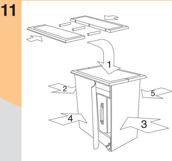
11 4200 Case Conversion: Latch the two cases together. Assemble top as shown and place on cases. Attach panels in numbered order shown. Velcro blotter to table top.
