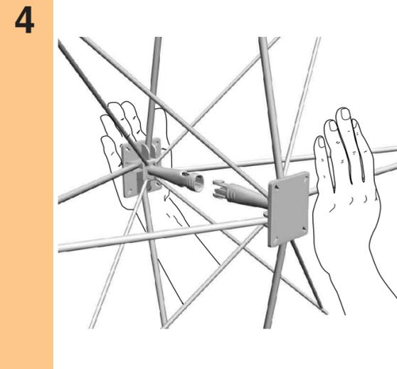
4 Ensure that spacer bars are fully engaged and locked.
