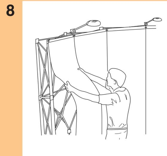
8 Release the panel, allowing it to attach magnetically to the channel bars. Straighten each panel by aligning it to the center of the channel bar slots.
