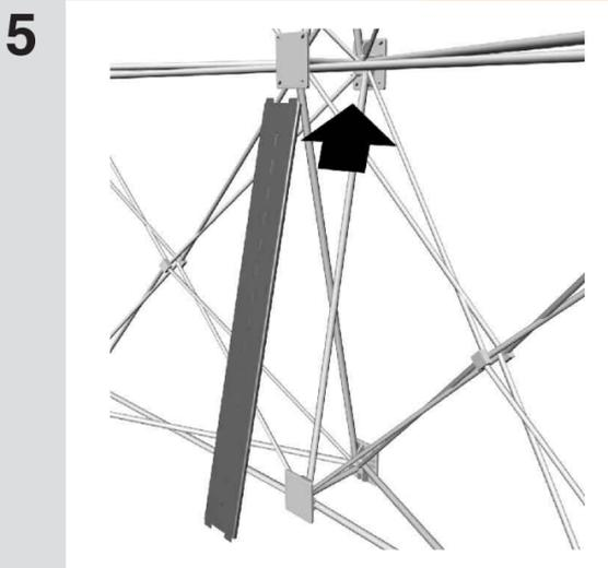
5 If applicable, attach stabilizer feet (not shown) to frame (refer to page 8 of Owner's Manual). Begin at the bottom center module and attach channel bars by sliding up onto the top hub.
