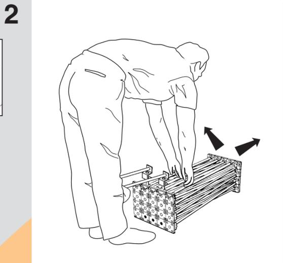
2 Grasp upper ends of frame and pull up and outward. Continue pulling up and outward until the frame is fully expanded. Spacer bars should be close enough to each other to allow for a connection.
